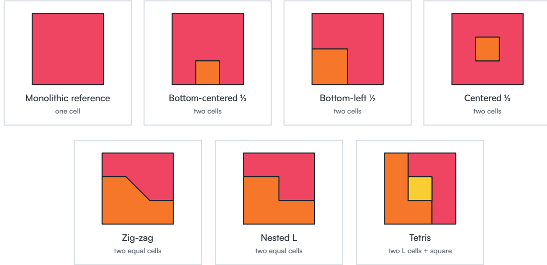
Figure 1: Normalized cross-sections used by the homogeneous material-interface study. Each color denotes a distinct retained cell and material definition; all material properties are identical.
