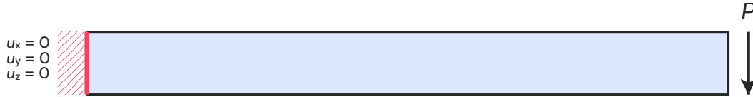
Figure 6: End-face shear traction represented by the resultant tip load P .
